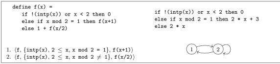
Fig. 1: Definition (top left), measure (top right), calling contexts (bottom left), and CCG (bottom right) for a function f.
