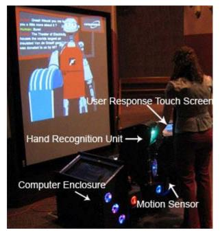
Figure 2. "Tinker" System Installation
