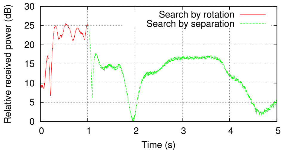
Figure 2.12: Fast: total received power relative to total received power’s minimum value during search.
