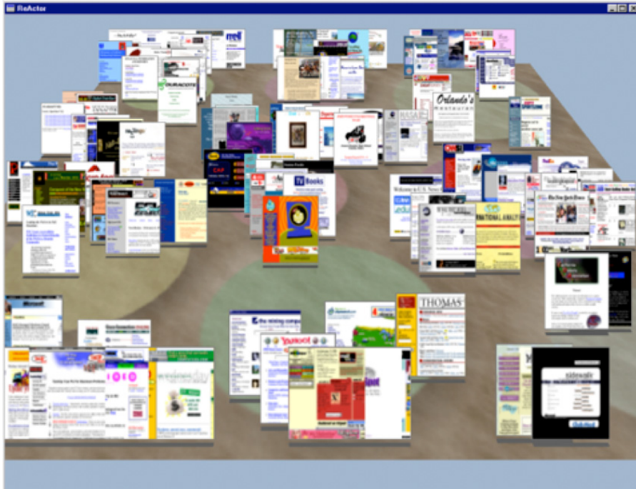
Fig. 3.30 Data mountain provides an inclined plane upon which web pages are organized (image from PDF).
