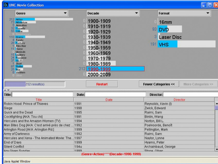
Fig. 3.6 The Relation Browser interface provides consistent facets, where the list of values is not filtered by selections. Instead, users can see (and preview by simply hovering) the reduction in files associated with each facet-value with the bar-chart style visualizations.
