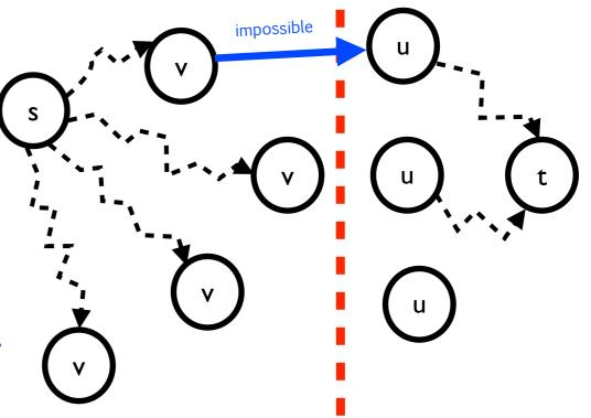
(c)=>(a): no flow can be bigger than capacity of a cut, so f must be a maximum flow (since it saturates the cut described above)
