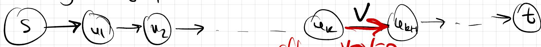
admit flow :  $\forall$  edge rev. capacity  $w(u_k, u_{k+1}) > 0$
