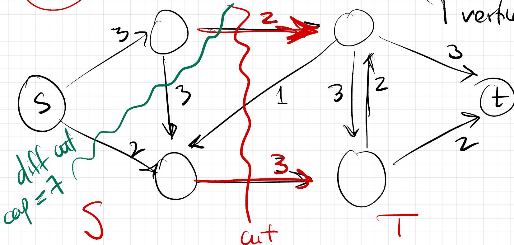
capacity of the cut  $S, T = \sum_{\substack{u \in S \\ v \in T}} W_{uv} = 2 + 3 = 5$
