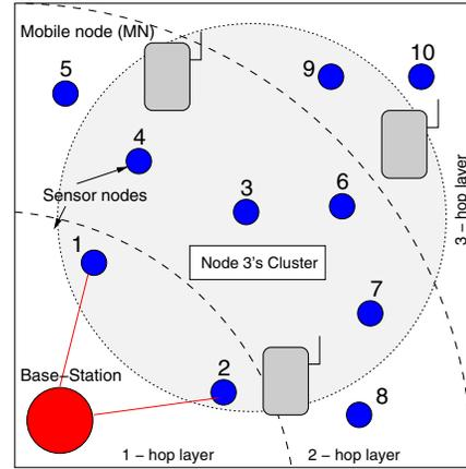
Fig. 1. Multi-hop infrastructure wireless sensor network architecture.
