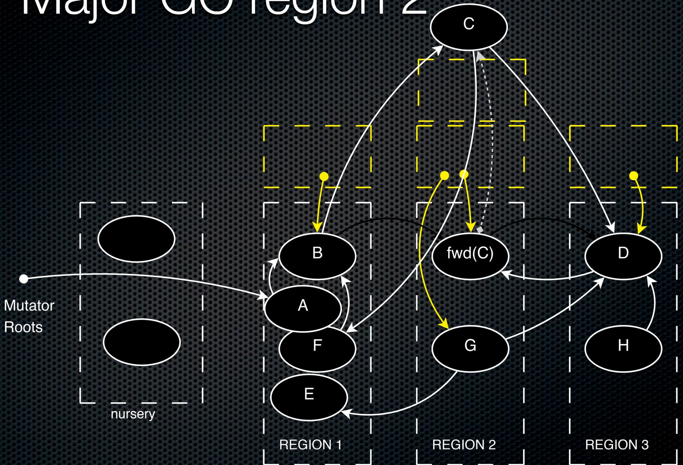
During the evacuation of C, we have to scan it for any objects it points to within region 2. That scan discovers region-crossing pointers, so C has to be kept in the new remembered set for region 2.
