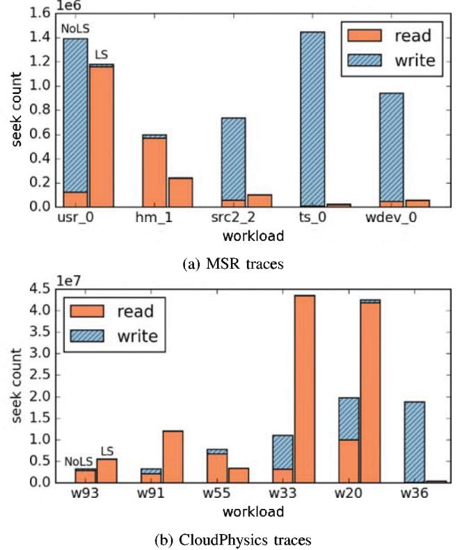
Fig. 2: Read and write seek counts of a subset of (a) MSR and (b) CloudPhysics traces for both non-log-structured (NoLS) and log-structured (LS) translation. We consider a seek to occur if an I/O operation starts at a sector other than that immediately following the previous operation.
