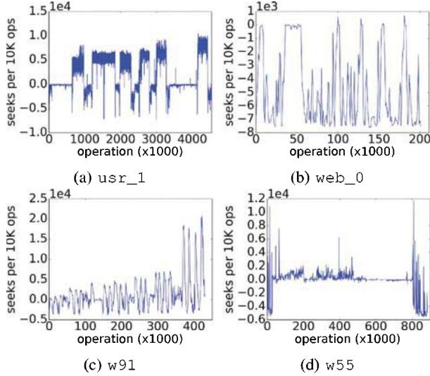
Fig. 3: Log-structured translation overhead (log-structured minus original) in terms of long ( $\geq 500\text{KB}$ ) seeks over time for MSR ((a) `usr_1` and (b) `web_0`) and CloudPhysics ((c) `w91` and (d) `w55`) workloads.
