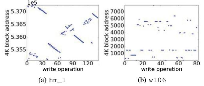
Fig. 7: Examples of highly non-sequential LBA accesses from traces (a) hm\_1 and (b) w106.
