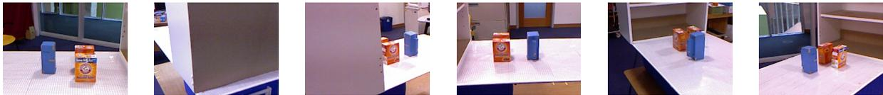
**Figure 3-9:** Examples of views from scenario 5. In all views except the final one, only one of the two orange baking-soda boxes was detected. This causes **MHT** to incorrectly infer that all measurements came from a single object (and prune other possibilities), whereas batch approaches such as clustering can revisit previous associations and correct them using new information, such as the final view where both boxes are finally detected.
