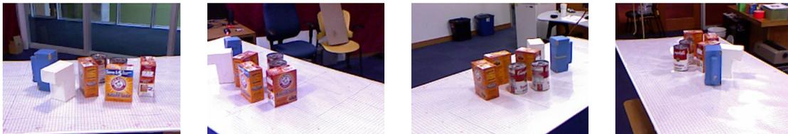
**Figure 3-10:** Examples of views from scenario 3. Objects were placed relatively close together, resulting in significant occlusion, causing the object detector to frequently miss detections or produce errors.
