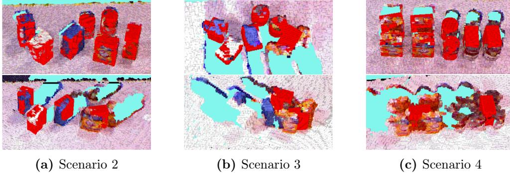
**Figure 3-8:** Examples of object detections in several views (superimposed in red using the known shape model of the detected type). The top row shows cases where the detections are relatively accurate, whereas the bottom row shows cases where most detections are missing or wrong. Missing objects are typically due to occlusion by other objects. When only a small part of an object is visible, it is often not segmented properly, which then affects the fitted poses.
