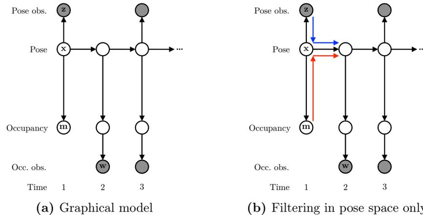
**Figure 5-9:** The generic filtering problem within a single representational layer.
