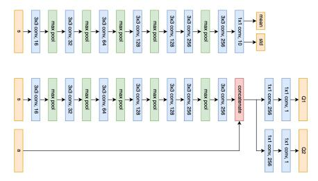
Figure 18: Network architecture of CNN SAC in robotic manipulation tasks.
