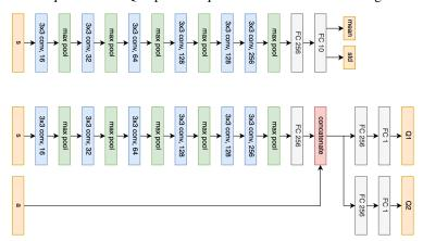
Figure 29: Network architecture of the 'fc1' variation for CNN SAC.
