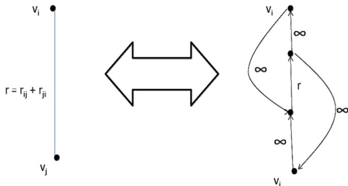
Figure 4: Bi-directional link with shared capacities and its corresponding gadget. Arc capacities are shown next to arcs.
