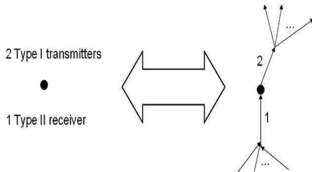
**Figure 1: Graph gadget that incorporates the radio restrictions at a node. Arc capacities are shown next to arcs.**
