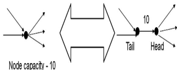
Figure 2: Transformation from node with capacity restriction on left to graph gadget on right. Node is split into a tail and a head with a capacity restriction on the intermediate arc.
