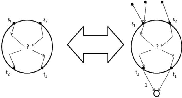
**Figure 5: Transformation from 2DIRPATH on left. Top three nodes at right are sources with demand 1. Except for left arc into the sink at bottom of capacity 1 rest have capacity 2. All nodes in the circle have radio constraint of at most one outgoing link.**
