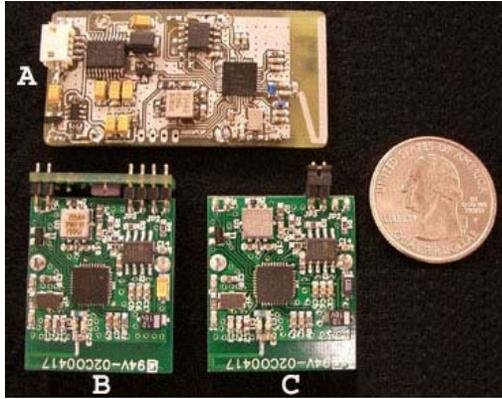
Figure 1. MITes: (A) receiver, (B) wearable accelerometer (3 axis, 10g), and (C) stick-on state-change (2 axis, 2g).
