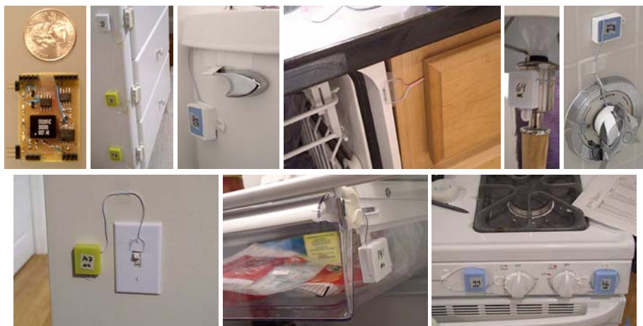
Fig. 2. The second tool is a system of environment state change sensors that can be installed ubiquitously throughout an environment such as a home. Each device consists of a data collection board and a small sensor, and the components are literally taped to objects and surfaces for the duration of the data collection period. These images show the data collection board outside of the protective case and 11 of the 85 sensors installed throughout one subject's home.
