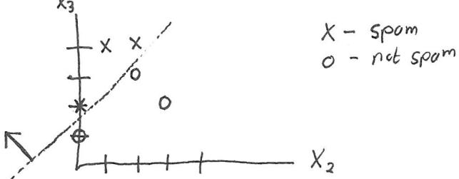
Observe we can separate  $x \& o$  with dashed line with slope 1 and  $X_3$ -intercept 1.5. ~~This is a linear classifier~~
