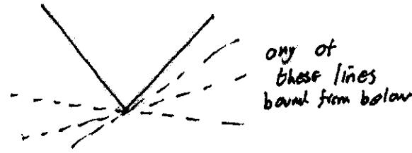
$v$  is subgradient of  $f: \mathbb{R}^n \rightarrow \mathbb{R}$  <sup>at  $y$</sup>  if  $f(x) - f(y) \geq \langle v, x-y \rangle \quad \forall x$
