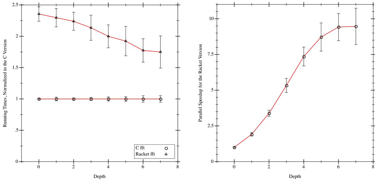
Figure 11: Comparison Between Racket and C and Parallel Speedup for Racket
