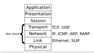
**Figure 1.** Layers of the OSI model and those implemented by  $S^3$
