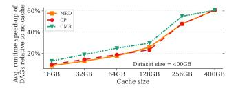
Figure 13: Mean runtime across all queries vs. cache size, normalized to uncached runtime; 10 Gb/s bandwidth. (simulated)
