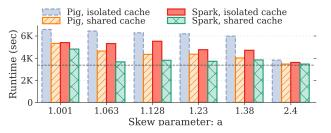
Figure 12: Performance of different frameworks with shared cache vs isolated cache per framework. Each cache has 1 TB cache, 25 Gb/s storage-bandwidth, and 100 Gb/s cache bandwidth. (simulated)
