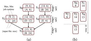
(a) (b) Figure 2: (a) 6-stage DAG divided into 3 stage-sets. Each stage is labeled with run-time (max=no input in cache, min=all input in cache), input file name and size. (b) Execution schedule with no prefetching or caching for gang-scheduling.
