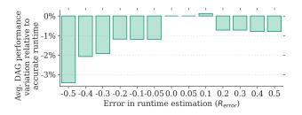
Figure 14: Sensitivity to misprediction error: introduced error vs. performance degradation - 30% of predications adjusted by factor of  $(1+R_{error})$ . (simulated)
