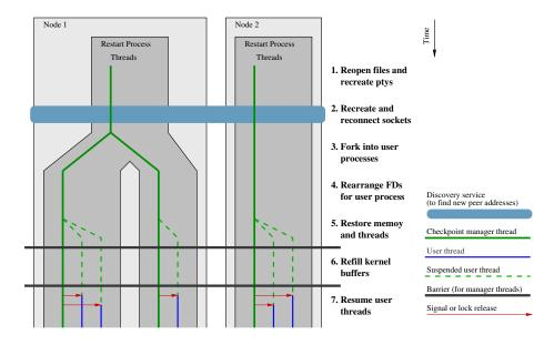
Figure 2: Steps for restarting the system checkpointed in Figure 1. The unified restart process and subsequent fork are required to recreate sockets and pipes shared between processes.
