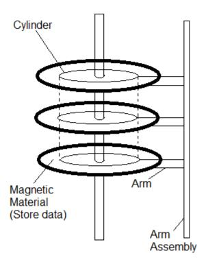
Above is a typical disk architecture. Where arms are of same locations and double sided (on both sides of a platter). There is a header at the end of the arm which is used to fetch data from platters.
