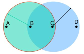
Hidden nodes: A and C send a packet to B; neither A nor C will detect the collision!
