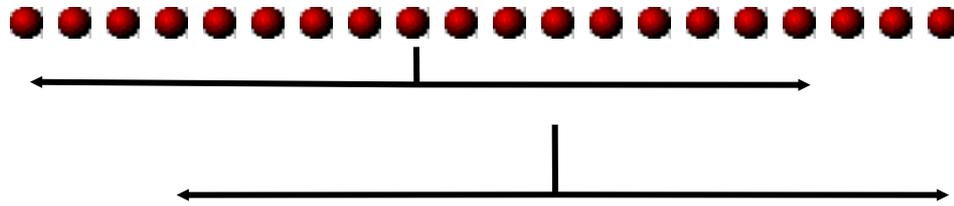
*Each node maintains IP addresses of the nodes with the  $L/2$  numerically closest larger and smaller nodeIds, respectively.*
