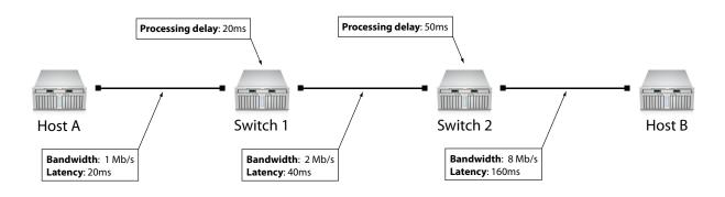
**1b.** (continuation of 1a) How much time does it take to transmit **two packets of size 1000 bytes** from Host B to Host A? You must show your work. *Hint: Because the bandwidths of the links are decreasing from Host B to Host A, the second packet will experience queuing delays in the switches.* (10 points)
