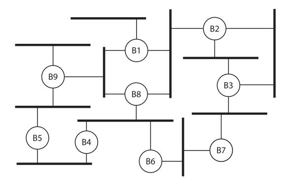
Indicate which ports are blocked by the bridge spanning tree protocol by putting an OXO over the corresponding ports. The bridge IDs are the numeric values. Feel free to label the ports with port numbers, if necessary. (15 pts)
