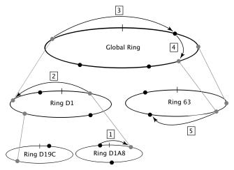
Figure 4: Diagram of a the routing process with multiple levels of hierarchy. Gray nodes are gateways, which exist in multiple rings and route between them. Numbers 1-5 denote the steps in routing.
