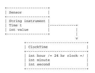
Figure 2: A class diagram for sensor readings
