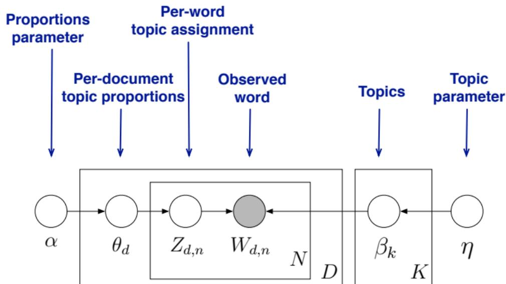
$$p(\beta, \theta, \mathbf{z}, \mathbf{w}) = \left( \prod_{i=1}^K p(\beta_i | \eta) \right) \left( \prod_{d=1}^D p(\theta_d | \alpha) \prod_{n=1}^N p(z_{d,n} | \theta_d) p(w_{d,n} | \beta_{1:K}, z_{d,n}) \right)$$
