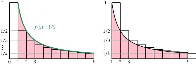
Figure 7.2: The  $k$ th harmonic number  $H_k = \sum_{i=1}^k 1/i$  is upper- and lower-bounded by two integrals. The value of these integrals is given by the area of the shaded region, while the value of  $H_k$  is given by the area of the rectangles.
