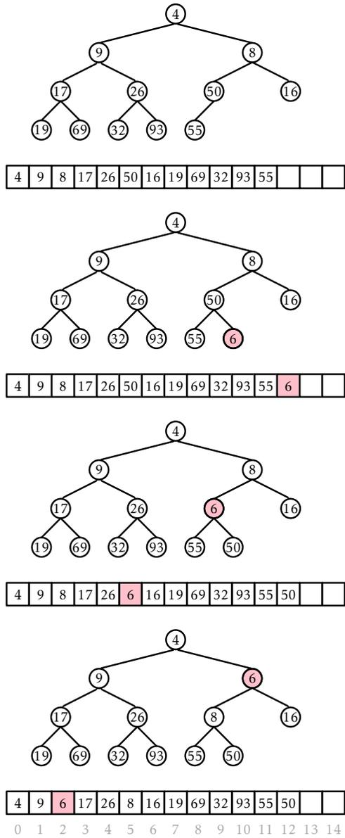
Figure 10.2: Adding the value 6 to a BinaryHeap.
