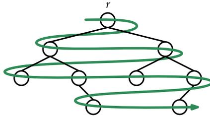
Figure 6.4: During a breadth-first traversal, the nodes of a binary tree are visited level-by-level, and left-to-right within each level.
