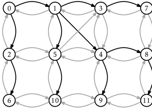
Figure 12.4: An example of bread-first-search starting at node 0. Nodes are labelled with the order in which they are added to  $q$ . Edges that result in nodes being added to  $q$  are drawn in black, other edges are drawn in grey.
