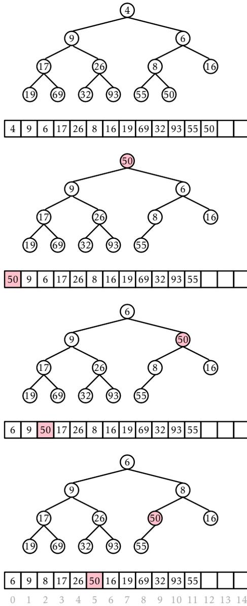
Figure 10.3: Removing the minimum value, 4, from a BinaryHeap.
