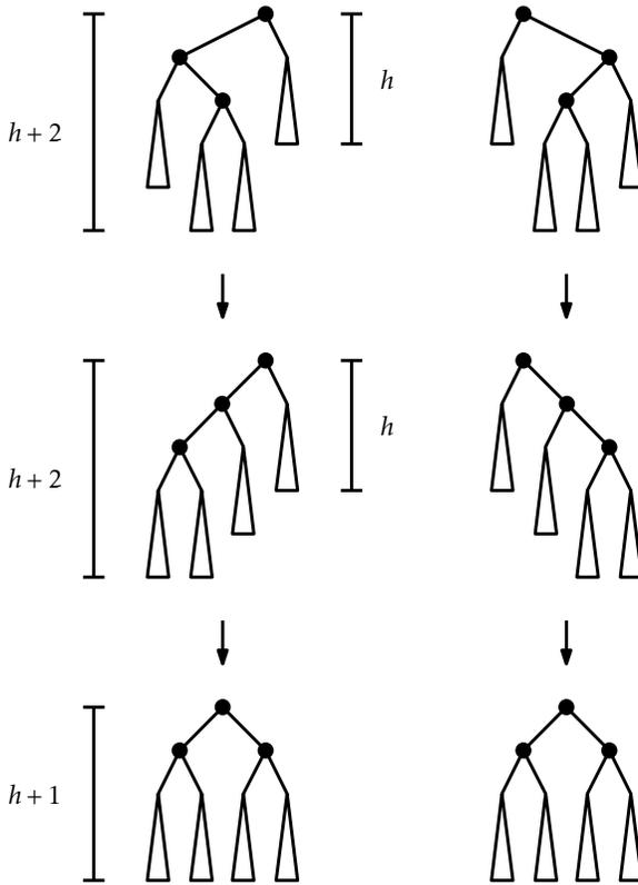
Figure 9.10: Rebalancing in an AVL tree. At most two rotations are required to convert a node whose subtrees have a height of  $h$  and  $h+2$  into a node whose subtrees each have a height of at most  $h+1$ .
