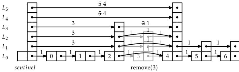
Figure 4.8: Removing an element from a SkiplistList.
