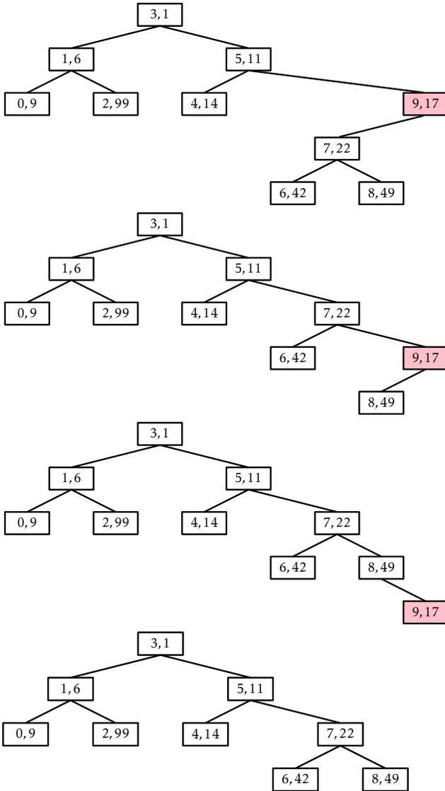
Figure 7.8: Removing the value 9 from the Treap in Figure 7.5.
