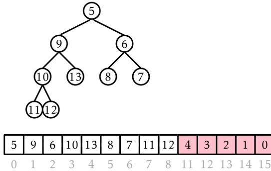
Figure 11.4: A snapshot of the execution of `heap_sort(a,c)`. The shaded part of the array is already sorted. The unshaded part is a `BinaryHeap`. During the next iteration, element 5 will be placed into array location 8.
