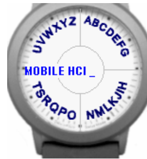
Figure 3: 5-button watch top text entry system (Dunlop, 2004).
