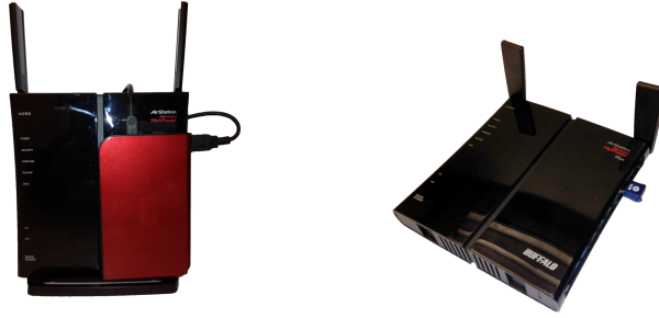
Figure 2: Open Infrastructure Testbed Prototype WiFi AP, Buffalo WZR-HP-G300NH, with 3.5" Hard Drive and 16GB USB Flash
