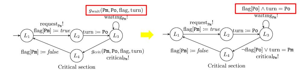
Algorithmic technique: counter-example guided completion of (extended) state machines
