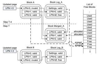
**Figure 9: Memorex device page update.** Using hybrid mapping and a full merge operation during garbage collection. LPN = Logical Page Number. LPN 2 is written to the log block of block B and the original LPN 2 marked invalid. If this requires a new log block, an old log block (Log\_A) must be freed by doing a merge with its corresponding data block.
