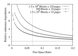
Figure 17: Degradation in performance due to wearleveling for uniformly-distributed page writes. The vertical line marks a free percentage of 6.7%, corresponding to usage of  $10^9$  out of every  $2^{30}$  bytes.
