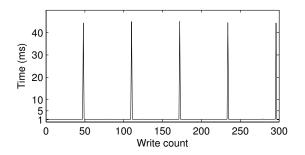
**Figure 10: House device write timing.** Write address is constant; peaks every 63 operations correspond to the merge operation (including erasure) described in Section 3.2.
