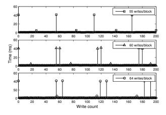
Figure 11: Memorex device garbage collection patterns. Access pattern used is  $\{A_1 \times n, A_2 \times n, ...\}$  for n = 55, 60, 64 writes/block.
