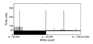
Figure 13: House device end-of-life signature. Latency of the final  $5 \times 10^4$  writes before failure.
