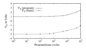
Figure 3: Typical  $V_T$  degradation with program/erase cycling for sub-90 nm flash cells. Data is abstracted from [24], [28], and [32].
