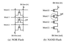
Figure 1: Flash circuit structure. NAND flash is distinguished by the series connection of cells along the bit line, while NOR flash (and most other memory technologies) arrange cells in parallel between two bit lines.
