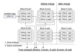
**Figure 8: House device single-page update.** Using hybrid mapping and a full merge operation during garbage collection. LPN = Logical Page Number. LPN 4 is written to block B, "shadowing" the old value in block A. On garbage collection, LPN 4 from block B is merged with LPNs 0 and 2 from block A and written to a new block.
