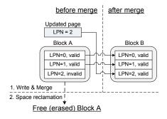
**Figure 7: Generic device page update.** Using block-level mapping and a partial merge operation during garbage collection. LPN = Logical Page Number. New data is merged with block A and an entire new block (B) is written.
