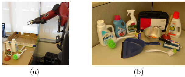
Fig. 6. (a) Typical grasping scenario. (b) The 12 objects used in our experiments. Notice that all objects have handles.
