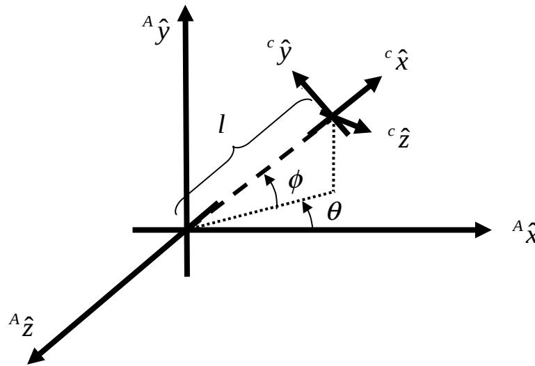
$${}^c d = \begin{pmatrix} -l \\ 0 \\ 0 \end{pmatrix} \quad {}^a d = -{}^a R_c {}^c d = - \begin{pmatrix} c_\theta c_\phi & -s_\phi c_\theta & s_\theta \\ s_\phi & c_\phi & 0 \\ -s_\theta c_\phi & s_\theta s_\phi & c_\theta \end{pmatrix} \begin{pmatrix} -l \\ 0 \\ 0 \end{pmatrix} = \begin{pmatrix} lc_\theta c_\phi \\ ls_\phi \\ -ls_\theta c_\phi \end{pmatrix}$$
