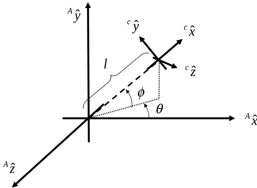
$${}^aR_c = {}^aR_b {}^bR_c = \begin{pmatrix} c_\theta & 0 & s_\theta \\ 0 & 1 & 0 \\ -s_\theta & 0 & c_\theta \end{pmatrix} \begin{pmatrix} c_\phi & -s_\phi & 0 \\ s_\phi & c_\phi & 0 \\ 0 & 0 & 1 \end{pmatrix} = \begin{pmatrix} c_\theta c_\phi & -s_\phi c_\theta & s_\theta \\ s_\phi & c_\phi & 0 \\ -s_\theta c_\phi & s_\theta s_\phi & c_\theta \end{pmatrix}$$
