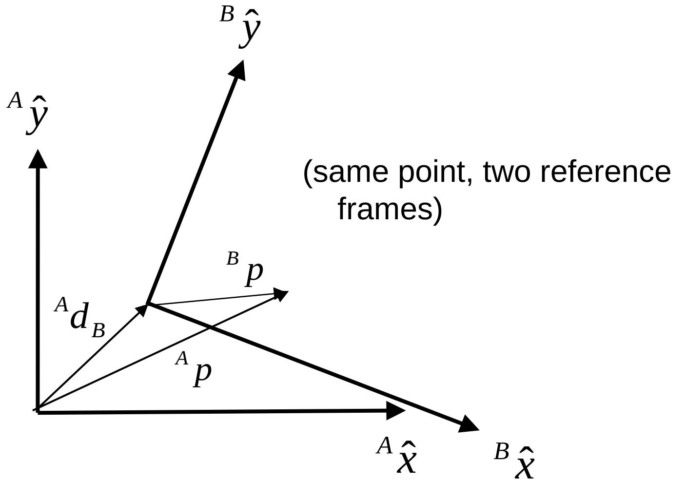
$$B p = {}^B R_A {}^A p - {}^B R_A {}^A d_B = {}^B R_A \left( {}^A p - {}^A d_B \right)$$
