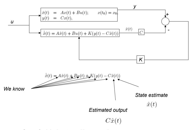
Copy of original system with a correcting term  $K(y(t) - C\hat{x}(t))$ which is the difference between the output and estimated output
