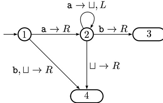
where 3 is the accept state and 4 is the reject state.
