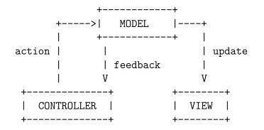
Roughly, the controller is in charge of directing the model by invoking actions, and the model informs the view when the state has changed so that the view can update its display (thus, the view is really an observer of the model). Often, the model sends feedback to the controller, because changes in the state of the application may change the possibilities open to the controller in terms of what actions can be performed.
