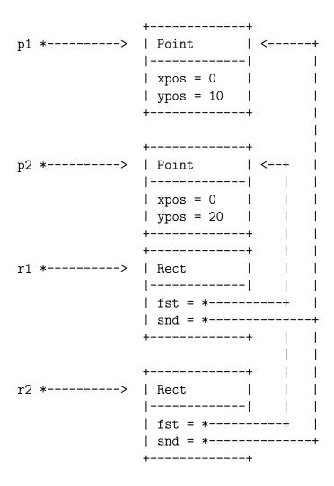
Which may not be *quite* what we want. It does create a fresh copy of r1, but since fst and snd are simply given the address of the object pointed to by fst and by snd are the same in both r1 and r2.
