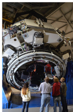
Lowell Discovery Telescope 4.3m Mirror. 36-megapixel CCD Happy Jack, AZ
