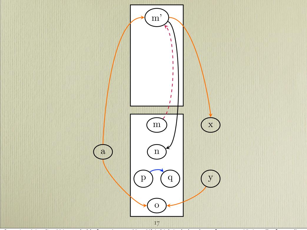
Scanning A implies M is reachable from A; copy M to M' (which includes that reference to N), install a forwarding pointer from M to M', and continue scanning A.
