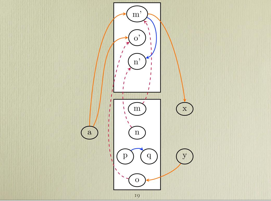
Scanning M' uncovers that reference to N; forward that to N'. Continuing left-to-right means scanning O' and N', which uncovers no more references within the region. So move on to the right side, where we have X and Y...
