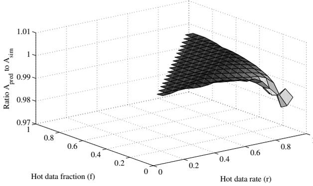
**Figure 9.** Ratio of predicted Greedy performance  $A_{pred}$  (Eq. 16) to simulated performance  $A_{sim}$  for  $S_f = 0.10$ ,  $N_p = 64$  across the range of values for  $r$  and  $f$ . For highly skewed data, relative error remains less than 2%.
