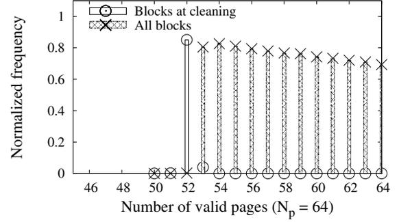
**Figure 3.** Greedy cleaning: distribution of block states (i.e. number of valid pages) overall and when selected for cleaning. Simulation parameters:  $S_f = 0.089$ ,  $N_p = 64$ ,  $U = 5 \times 10^4$
