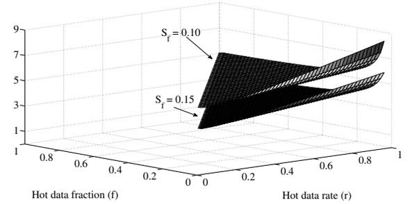
**Figure 8.** Performance of LRU cleaning with mixed hot/cold traffic for different values of  $r$  and  $f$ , for  $S_f = 0.1$  (upper graph) and  $S_f = 0.15$  (lower one). As  $r \rightarrow 1$  and  $f \rightarrow 0$ , write amplification increases from 5.2 to 8.4 and from 3.5 to 5.9, respectively.
