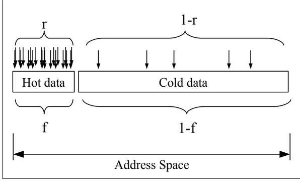
**Figure 5.** Hot/Cold data model used for analysis. The fraction of the total write rate destined for “hot” pages is  $r$ ; these hot pages represent a fraction  $f$  of the overall address space—e.g. 80% of writes destined to 20% of the address space..
