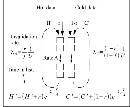
**Figure 7.** Balance equations for LRU cleaning with hot/cold traffic. At each step (i.e. external write) the odds of a hot page being invalidated are  $\frac{r}{fU}$ ; during a block’s passage through the list the number of external writes is  $\frac{T}{A}$ .
