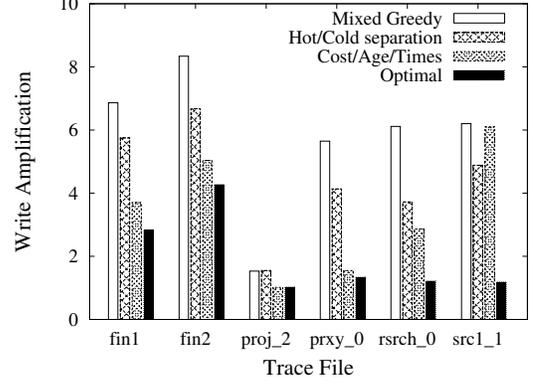
**Figure 15.** Write amplification for write-only storage traces using global greedy, greedy with hot/cold separation, linear CAT metric hot/cold separation, and optimal cleaning;  $N_p = 64$ ,  $S_f = 0.07$ .
