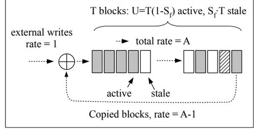
**Figure 1.** Model of LRU block cleaning. External writes enter at rate 1; blocks move through the queue at rate  $A$ , and are invalidated at a rate of  $\frac{1}{U}$ ; at the end of the queue they thus remain valid with probability  $(1 - \frac{1}{U})^{T/A}$ , which must also be equal to  $\frac{1}{A-1}$ .
