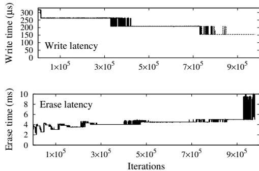
**Figure 5: Wear-related changes in latency.** Program and erase latency are plotted separately over the lifetime of the same block in the 8Gb MLC device. Quantization of latency is due to iterative internal algorithms.
