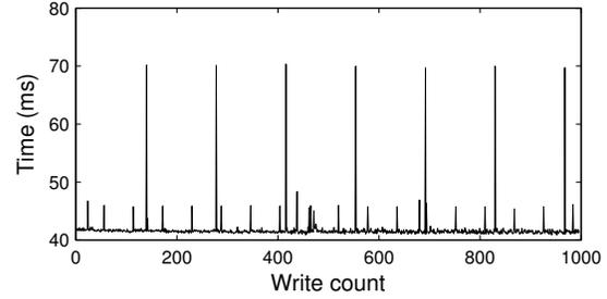
**Figure 12: Memorex device static wear-leveling.** Lower values represent normal writes and erasures, while peaks include time to swap a static block with one from the free list. Peaks have a regular frequency of one at every 138 write/erase.
