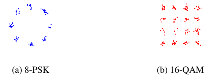
Figure 1: Constellation guessing on USRP: Received symbols can be distinguished clearly after carrier synchronization and tracking.
