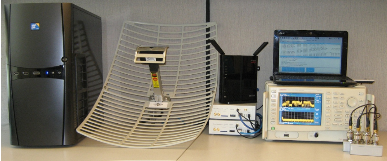
Figure 5. Overview of hardware used in the prototype implementation of the attack. From left: desktop, antenna, router, USRP2 software-defined radio, victim client, signal analyzer (for evaluation), and attenuators.
