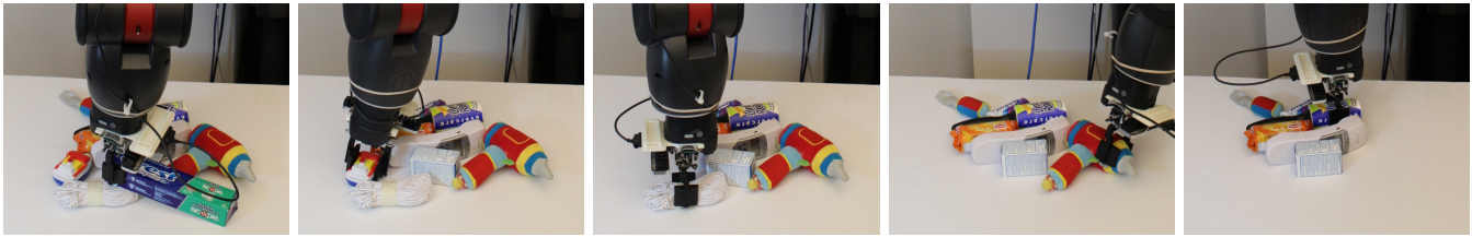
Fig. 10. First 5 grasps of a typical experiment trial. All grasps were successful. This was a run with all 3 views included.
