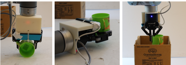
Fig. 1. Illustration of pick and place scenario that requires multiple picks and places. (Left) Object is grasped in initial configuration. (Center) First place is to make the mug upright so it can be grasped from the top. (Right) Places mug deep in box – the gripper must be vertical to box.
