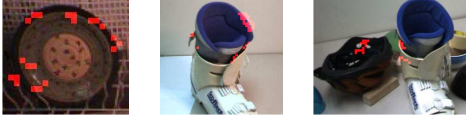
Figure 3.4: Sample outputs from image-based classifiers. Red patches indicate the predicted grasping points.
