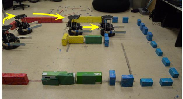
Fig. 1: In this robot demonstration we provided a natural language command of “Go through the yellow room to the blue room”. The command is mapped to the LTL formula  $\diamond(Y \wedge \diamond B)$ , which implies eventually satisfying the combination of going to yellow and subsequently reaching the blue room. In this work we map from natural language commands to such LTL formulae with sequence-to-sequence approaches.
