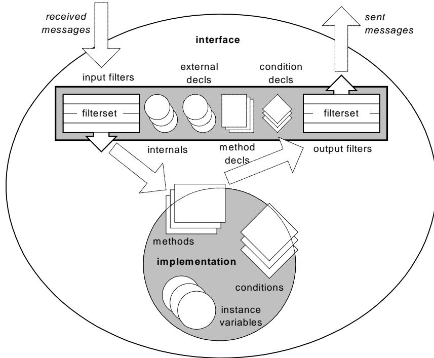
Figure 5. Simplified representation of the CF model.
